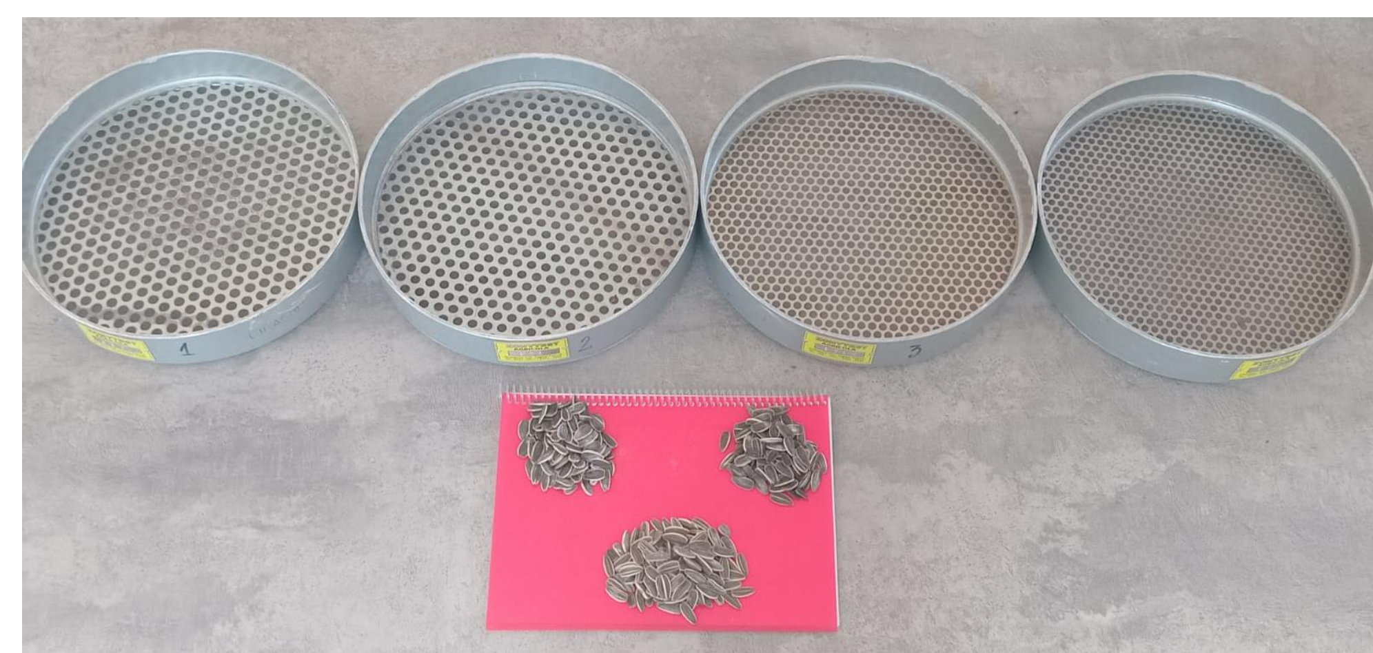
Figure 2. View of four-mesh sieve: 9.5 mm, 8.75 mm, 8 mm and 6.5 mm. respectively and three hybrids of this study.
