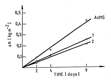
Fig. 1. Water vapour permeability of films on the basis of acetylated monoacyl glycerol (AcMG) with the addition of sunflower oil waxes 1 - 92% AcMG + 8% SW 2 84% AcMG + 16% SW
