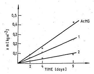
Water vapour permeability of films on the basis of acetylated monoacyl glycerol (AcMG) with the addition of bees waxe (BW) 1 - 92% AcMG + 8% SW 2 - 84% AcMG + 16% SW Fig. 2.
